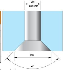
The **UCHAMF inserts** are offered as standard (82°, 90° countersink angles) or semi-standard solutions tailored to meet customer-specific applications. It is mandatory to match the tool-holder series with the corresponding insert series.
